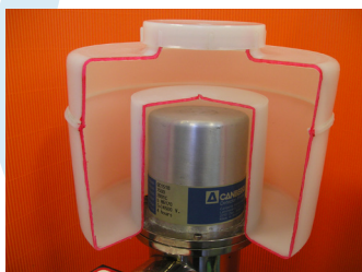
Left: Cross-section of a Marinelli™ beaker on a Ge-detector. Right: Source preparation using pycnometer vials.
