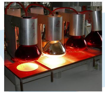
Right: Evaporation of water samples for gross alpha/beta counting.
