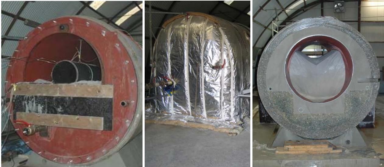
Grout backfilling tests: mock-up with central heater (left) and insulation (centre). Perfect filling of the gap was illustrated when a slice of the mock-up was cut (right).
