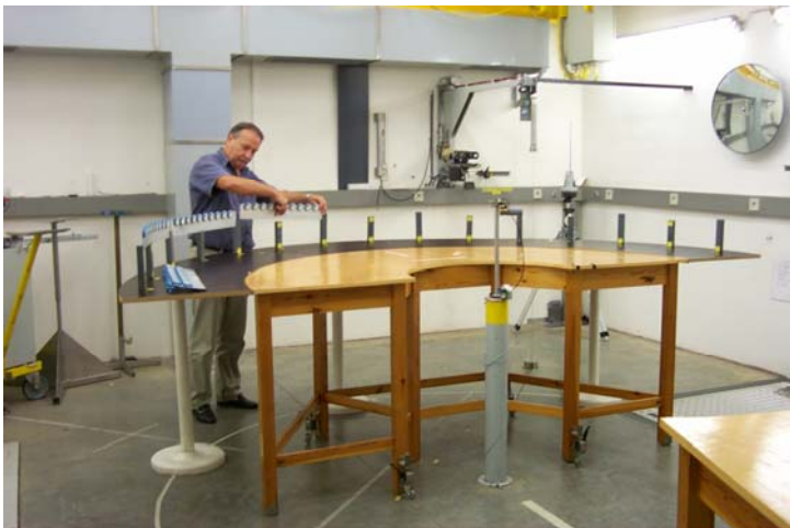
Figure 2: Preparation of doseimeters for panoramic irradiation
