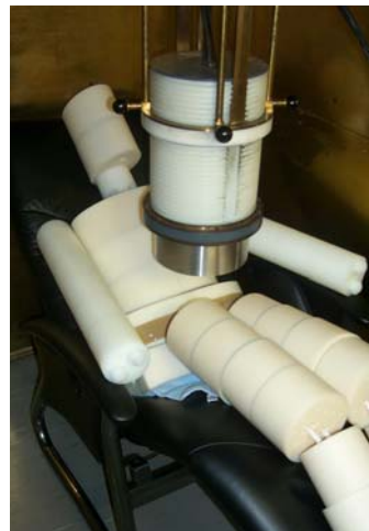
Figure 3: Setup for calibration of WBC system with modular nylon phantom and NaI detector.
