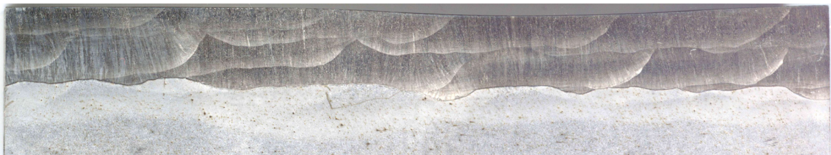
Macrograph of the cladding. From bottom to top three zones can be identified: base material, first layer and second layer. Total cladding thickness is about 9 mm.
