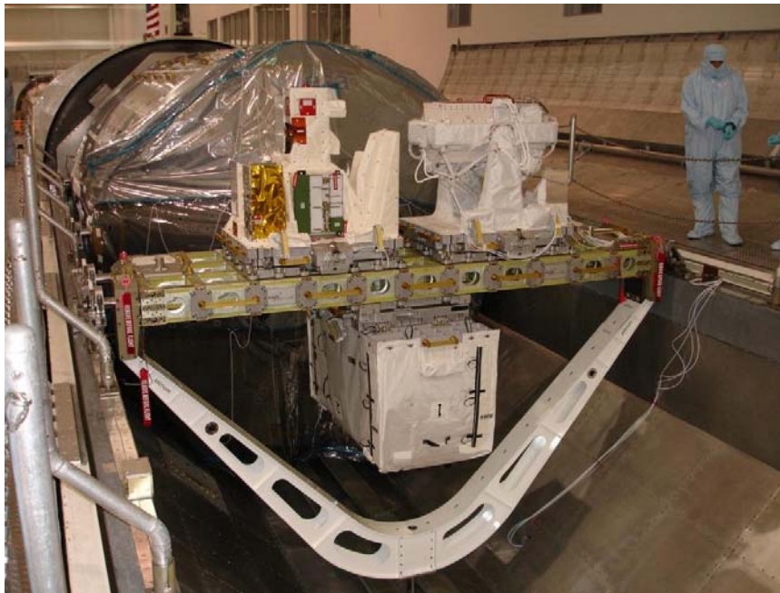
The EXPOSE-EUTEF module ready to be integrated in the Atlantis Space Shuttle
