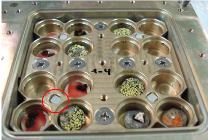
Thermoluminescent detectors of SCK•CEN integrated in the experimental trays of the EXPOSE-EUTEF module
