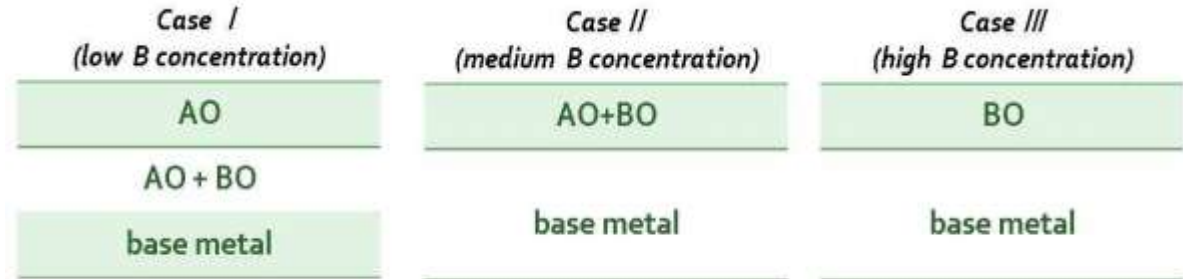
Schematic models of the general scale growth on A-B alloys
