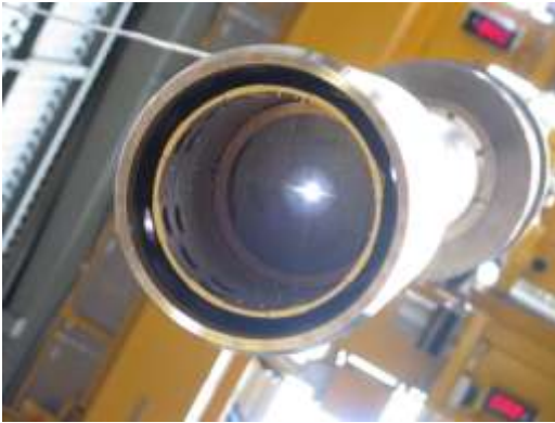
VIMOS: beam footprint visualization system
