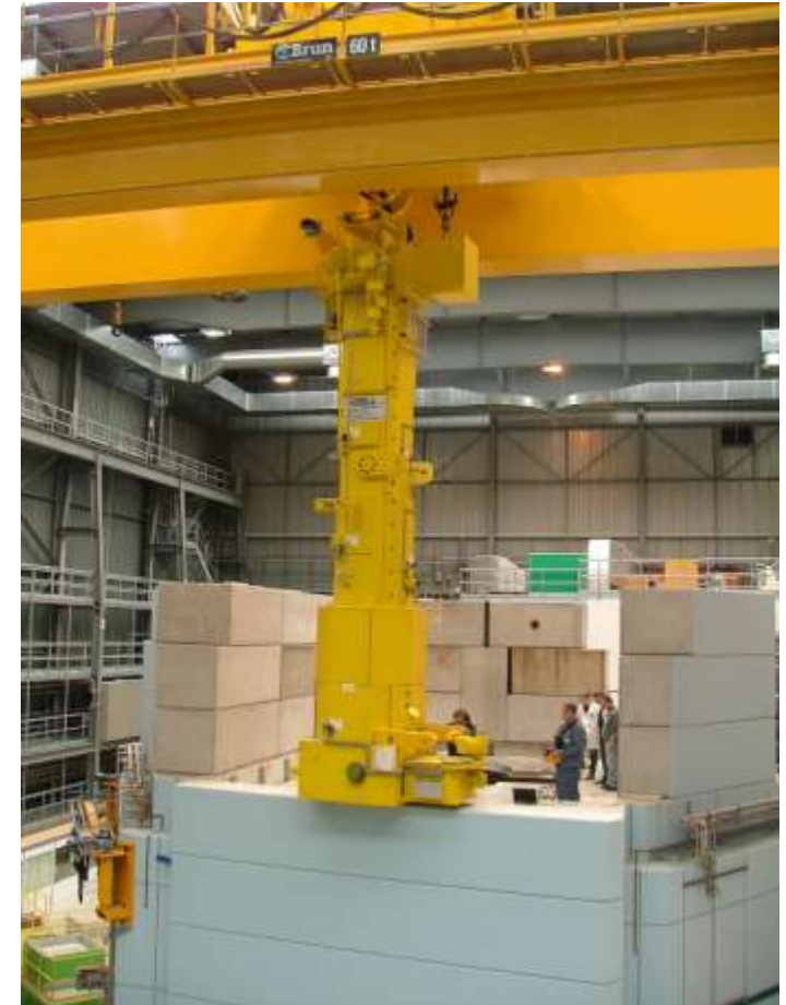
inserting the target into SINQ with the exchange flask
