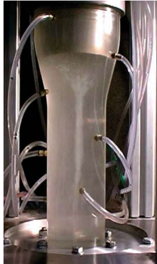
Flow visualization at 10 l/s for a swirl intensity of 10.5%
