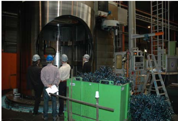
Reinforcement structure: milling of the structure as a whole (left) and assembly underground (right)
